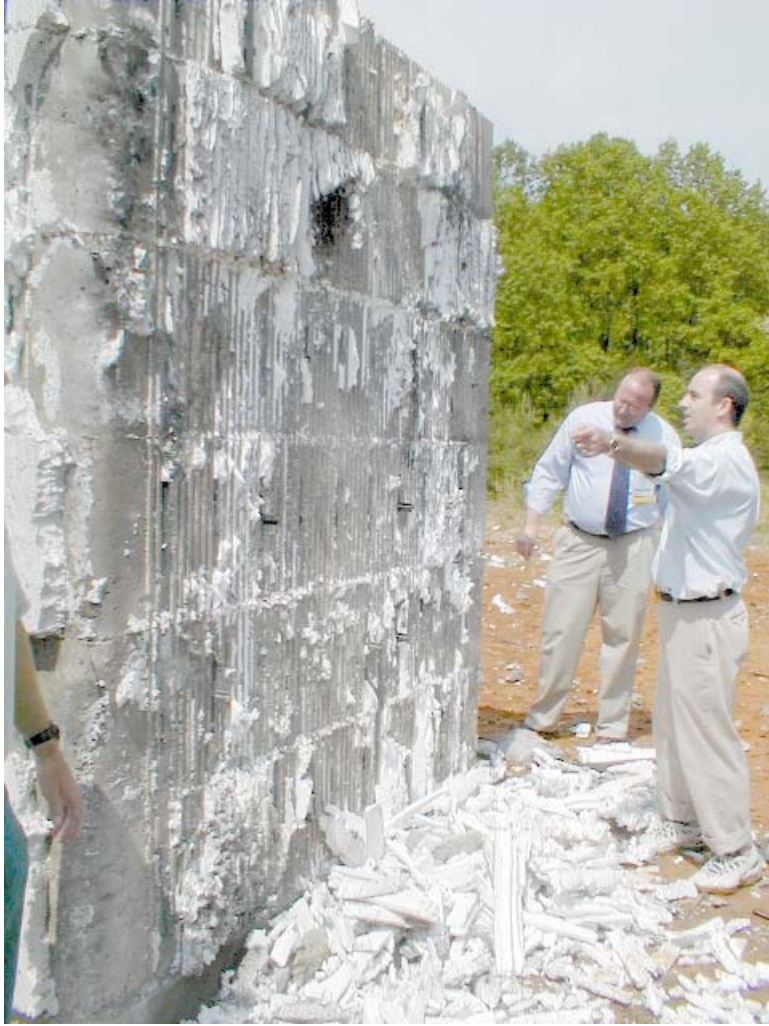
Figure 6 – Evaluation of Specimen E after the EPS was manually removed to expose the underlying
