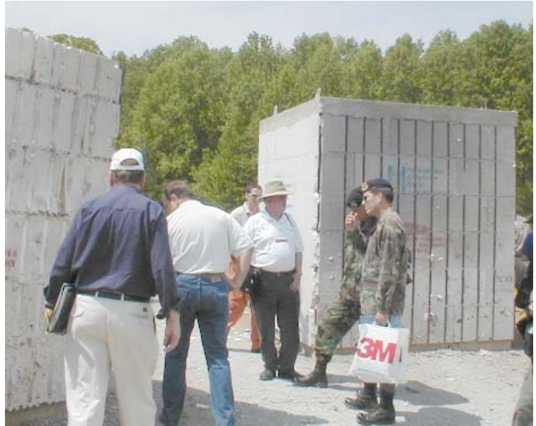
Figure 4 – Specimens C (left) and D (right). Signs of compression of the EPS can be seen in the wall facing the blast of Specimen D. (Note how the ribs are only seen on the side facing the blast.) Embedded shrapnel can be seen on the bottom of Specimen D. Also, although exposed, no damage was seen to the edge of the upper slab.
